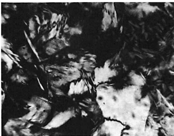
Fig. 6. Mesomorphic-like and crystalline phases of polymer I observed on cooling.
